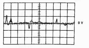
VERT DEF 10 V PER DIV HORZ DEF 1 US PER DIV SYNC TIME ØØØ TEST POINT FO4A TO FO8A LOGIC 425711 COMMENT OPEN DIVERTER CARD
