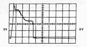
VERT DEF 10 V PER DIV HORZ DEF 1 US PER DIV SYNC TIME ØØØ TEST POINT FØSA OR FOBA (R1 TIME) LOGIC 425711 COMMENT SHORTED CURRENT SOURCE ENTER KEY UP
