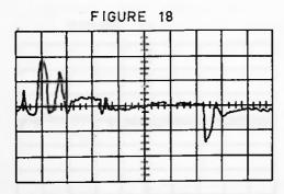
VERT DEF 10 V PER DIV HORZ DEF 1 US PER DIV SYNC TIME ØØØ TEST POINT F04C OR F07C LOGIC 425711 COMMENT 2 DECODES CONDUCTING (1 SHORTED)
