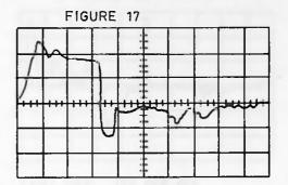
VERT DEF 10V PER DIV HORZ DEF 1 US PER DIV SYNC TIME ØØØ TEST POINT FOSC OR FO8C LOGIC 425711 COMMENT NO DECODE SWITCH CONDUCTING
