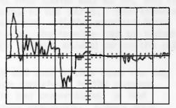
VERT DEF 10V PER DIV HORZ DEF 1 US PER DIV SYNC TIME Ø Ø TEST POINT UNITS 1 (E 13P) LOGIC 425311 COMMENT DECODE SWITCH NORMALLY NOT CONDUCTING
