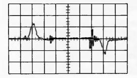
VERT DEF 0,05V BOTH CHANNELS DIRECT PROBES HORZ DEF 1 US PER DIV SYNC TIME ØØØ TEST POINT 01A1D04A AND C LOGIC 42.59.1.1. COMMENT FERRITE CORE SENSE LINE RESPONSE (MODE ADDED WITH ONE CHANNEL INVERTED) 17. -
