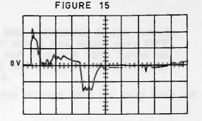
VERT DEF 10 V PER DIV HORZ DEF 1 US PER DIV SYNC TIME ØØØ TEST POINT FØ5C OR FØ8C LOGIC 425711 COMMENT CORRECT OUTPUT OF DIVERTER WHEN ONE DECODE IS CONDUCTING (ENTER SWITCH ON )
