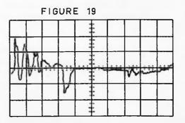
VERT DEF 10 V PER DIV HORZ DEF 1 US PER DIV SYNC TIME ØØØ TEST POINT F05C OR F08C LOGIC 425711 COMMENT 2 DECODES CONDUCTING (1 SHORTED )
