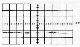
VERT DEF 10 V PER DIV HORZ DEF 1 US PER DIV SYNC TIME ØØØ TEST POINT F04A TO F08A LOGIC 425711 COMMENT SHORTED DIVERTER CARD
