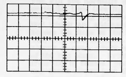
VERT DEF 5 V PER DIV HORZ DEF 1 US PER DIV SYNC TIME ØØØ TEST POINT F 19G (BIT 2) STAGE 2 LOGIC 425811 COMMENT OUTPUT OF INHIBIT DRIVER (NOT CONDUCTING) BIT ENTERED
