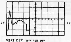
HORZ DEF 1US PER DIV SYNC TIME Ø Ø Ø TEST POINT FOSA OR FORA (R1 TIME) LOGIC 425711 COMMENT CORRECT CURRENT SOURCE
