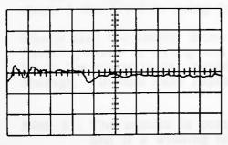
VERT DEF 10 V PER DIV HORZ DEF 1 US PER DIV SYNC TIME ØØØ TEST POINT UNITS Ø (E13E) LOGIÇ 425311 COMMENT SHORTED DECODE ALWAYS CONDUCTING (NOT ADDRESSED) FIGURE 21
