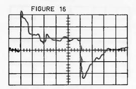
VERT DEF 10 V PER DIV HORZ DEF 1 US PER DIV SYNC TIME ØØØ TEST POINT F04C OR F07C LOGIC 425711 COMMENT NO DECODE SWITCH CONDUCTING
