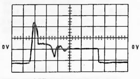
VERT DEF 10 V PER DIV HORZ DEF 1 US PER DIV SYNC TIME Ø Ø Ø TEST POINT FO4A CR3TIMED LOGIC 425711 COMMENT CORRECT CURRENT SOURCE FIGURE 4
