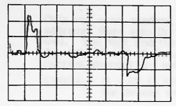
VERT DEF 10V PER DIV HORZ DEF 1US PER DIV SYNC TIME ØØØ TEST POINT F04C OR F07C LOGIC 425711 COMMENT CORRECT OUTPUT OF DIVERTER WHEN ONE DECODE IS CONDUCTING CENTER SWITCH ON )
