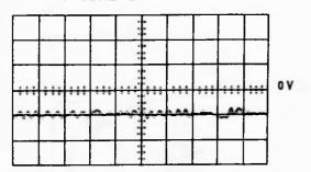
VERT DEF 5V PER DIV HORZ DEF 1 US PER DIV SYNC TIME ØØØ TEST POINT FO4A TO FO8A LOGIC 425711 COMMENT SHORTED CURRENT SOURCE ENTER KEY DOWN
