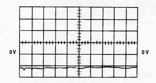
VERT DEF 10 V PER DIV HORZ DEF 1 US PER DIV SYNC TIME \$ \$ \$ TEST POINT FOSA OR FORA (R1 TIME) LOGIC 425711 COMMENT OPEN CURRENT SOURCE ENTER KEY UP
